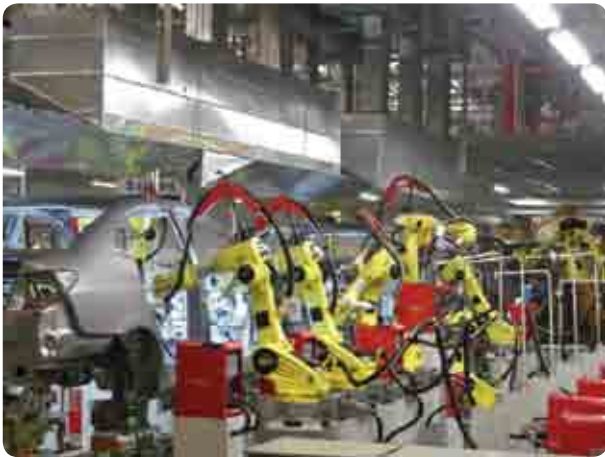
Arc welding robot
